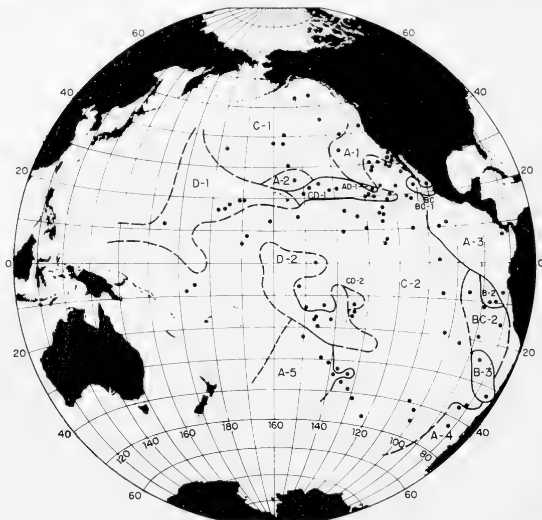
Fig. 6. Regional variation in chemical composition of manganese nodules. Regions marked A are characterized by ratios Mn/Fe less than 1; B-areas conversely have exceptionally high ratios Mn/Fe (ranging from 12 to 50). In areas marked C the nickel and copper content of the nodules is unusually high. D denotes regions with large amounts of cobalt (0.7–2.1%) in the nodules. (Mero, unpublished, modified from Mero, 1960a.)
